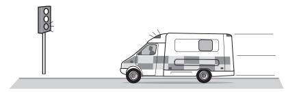
The ambulances used by the health authority are fitted with RFID chips. These are scanned when the ambulance approaches traffic signals. If the ambulance is on an emergency call the lights automatically change to green.
