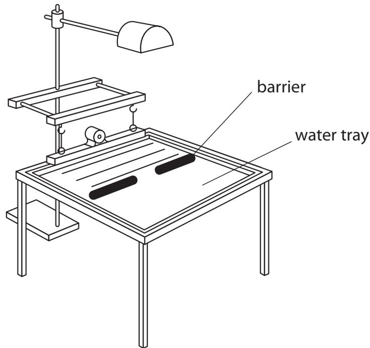
The ripple tank produces plane waves.
