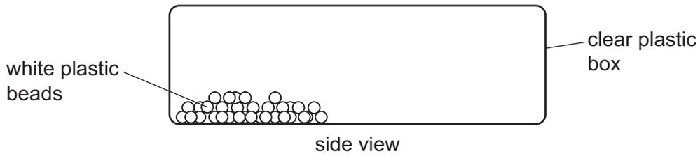
The box is shaken and the beads rub against the box. The beads stick to the inside surface of the box.
