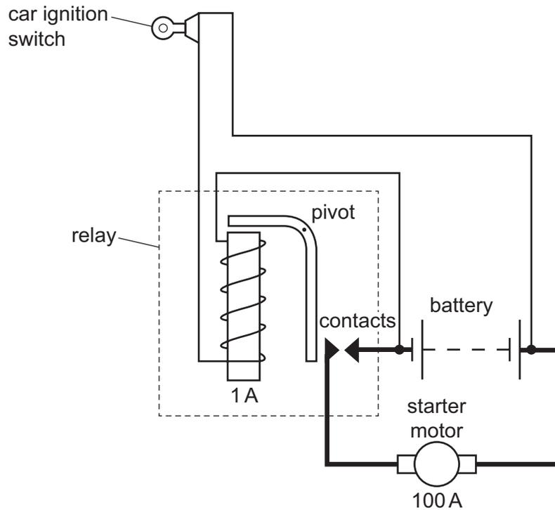
The ignition switch is in a circuit with long, thin wires. The starter motor is in a circuit with short, thick wires.
