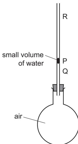
When the flask is held in a student's hands, the small volume of water first moves down from P to Q, and then up to R.
