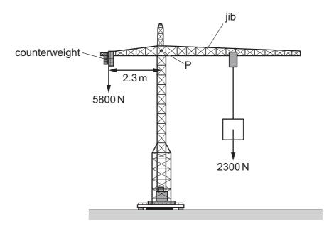
What is the horizontal distance between the 2300 N load and P so that there is no moment about P?
