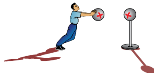
Figure 23.6 Work must be done to push one positive charge towards another.
