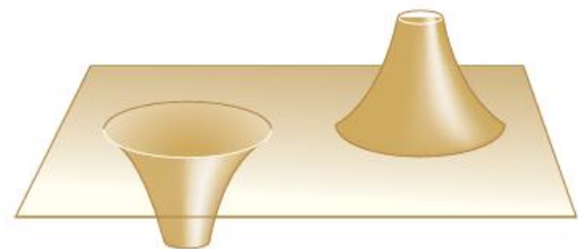
Figure 23.12 A 'potential well' near a negative charge, and a 'potential hill' near a positive charge.
