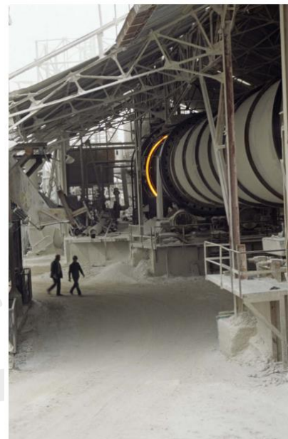
Figure 11.8 In a rotating lime kiln, calcium carbonate undergoes thermal decomposition to form calcium oxide and carbon dioxide.
