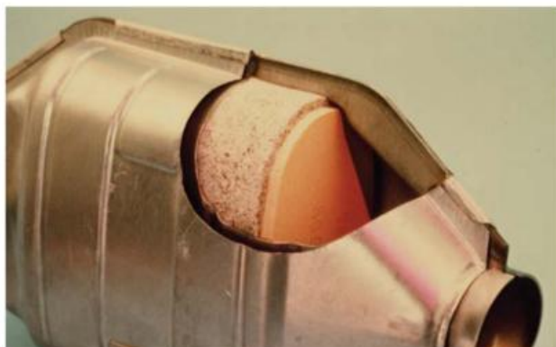
Figure 15.9 Catalytic converters reduce the pollutants from car exhausts. Precious metals, such as platinum, are coated on a honeycomb structure to provide a large surface area on which the reactions can occur.
