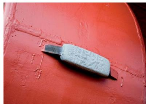
Figure 7.2 This is part of a ship's hull. It is made of iron protected by bars of magnesium metal. The magnesium atoms (oxidation number = 0) are oxidised to \text{Mg}^{2+} ions (oxidation number = +2) in preference to iron atoms changing to \text{Fe}^{3+} . This is called sacrificial protection.
