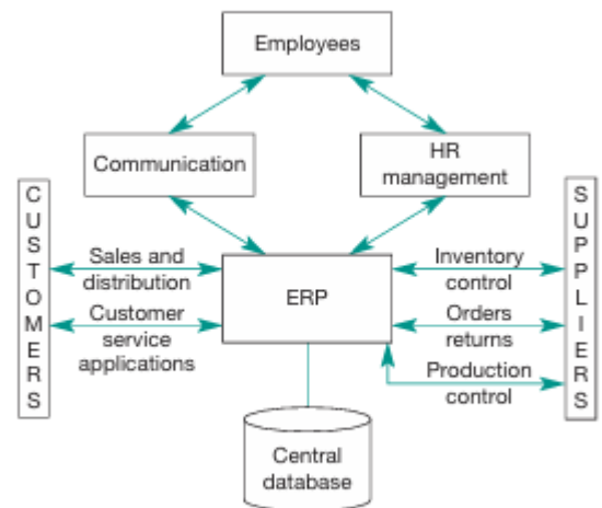
Figure 23.2 Enterprise resource planning uses a company-wide computer software system to manage resources
