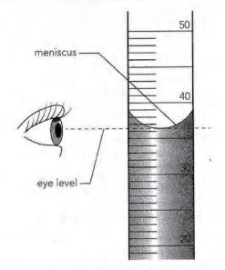
Figure 22.14: How to take an accurate burette reading.
