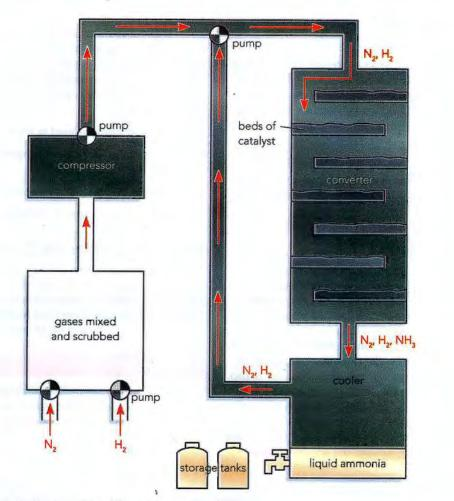
Figure 9.11: A schematic drawing of the different stages of the Haber process.
