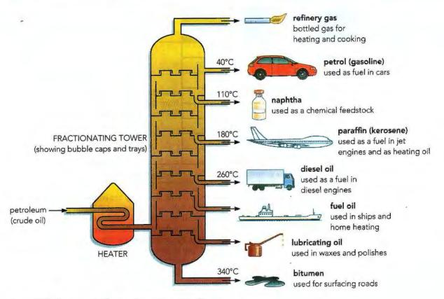
Figure 20.3: Fractional distillation of petroleum in a refinery.
