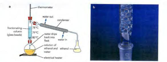
Figure 21.12 a: Separating a mixture of ethanol (alcohol) and water by fractional distillation. b: A close-up of the glass beads in the fractionating column.
