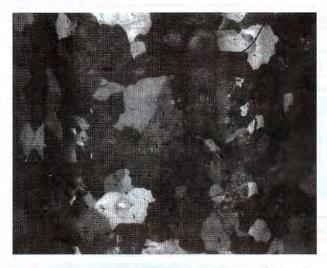
Figure 16.11: A photograph of zinc grains on a galvanised fence post.
