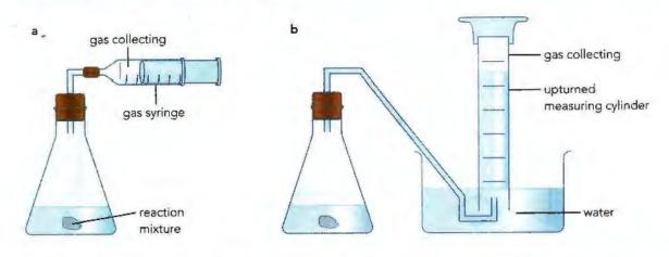
Figure 21.5: Collecting and measuring the volume of a gas: a: in a gas syringe and b: over water in an inverted measuring cylinder.
