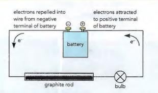
**Figure 6.3:** Testing a solid material (a graphite rod) to see if the material conducts electricity. The bulb will light if the material is an electrical conductor.
