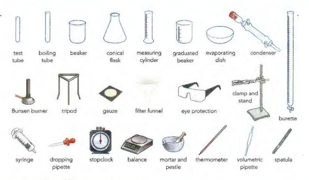
Figure 21.3: Common laboratory equipment.
