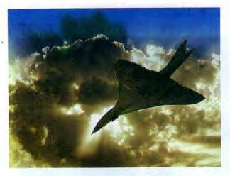
**Figure 14.10:** The world's first supersonic passenger jet *Concorde* was built out of an alloy containing over 90% aluminium.
