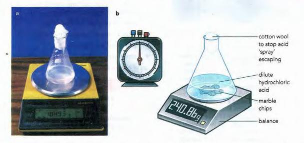
Figure 8.6: Apparatus for experiments A and B: the reaction of marble chips with dilute hydrochloric acid. The loss of carbon dioxide from the flask produces a loss in mass. This is detected by the balance.
