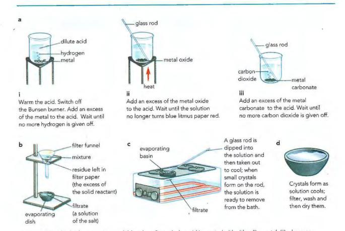
**Figure 12.8:** Method A for preparing a soluble salt. **a:** Stage 1: the acid is reacted with either (i) a metal, (ii) a base or (iii) a carbonate. **b:** Stage 2: the excess solid is filtered out. **c:** Stage 3: the solution is carefully evaporated. **d:** Stage 4: the crystals are allowed to form.
