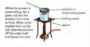
Figure 21.10: Evaporation method to produce the salt crystals.
