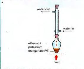
Figure 19.22: Oxidation of ethanol with acidified potassium manganate(VII) under reflux.
