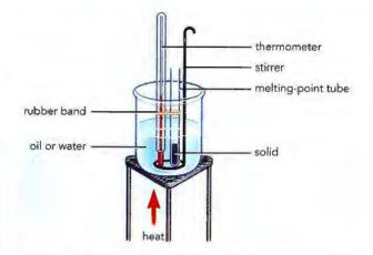
**Figure 1.9:** Apparatus for measuring the melting point of a solid. A water-bath can be used for melting points below 100 °C and an oil bath for melting points above 100 °C.
