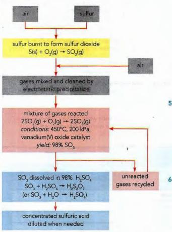
Figure 9.14: Flow chart for making sulfuric acid by the Contact process.
