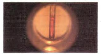
Figure 21.13 b: Magnified view through a lens of a sample being analysed for its melting point in a melting point apparatus.
