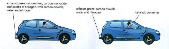
Figure 17.5: A catalytic converter converts harmful exhaust gases into safer gases.
