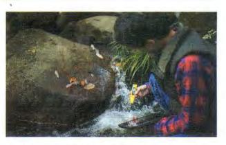
Figure 21.4: Digital pH meter being used by a research scientist to test water quality.
