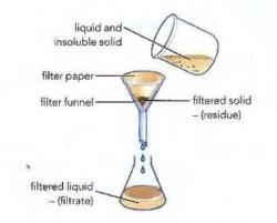
**Figure 21.9:** Filtration to remove the insoluble components of the rock salt mixture.
