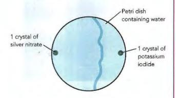
Figure 1.22: Experiment to investigate diffusion through water.
