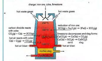
Figure 16.6: Key reactions of the extraction of iron and the regions of the blast furnace where they take place.
