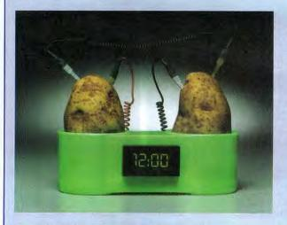
Figure 15.1: A potato-powered digital clock.
