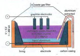
Figure 16.8: Electrolytic cell for extracting aluminium.
