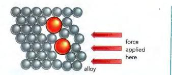
Figure 14.15: Alloys are stronger than pure metals because the layers cannot slide over each other easily as in a pure metal.
