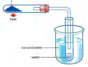
Figure 9.2: Apparatus for condensing the water vapour driven off from blue crystals of hydrated copper(II) sulfate by heating.
