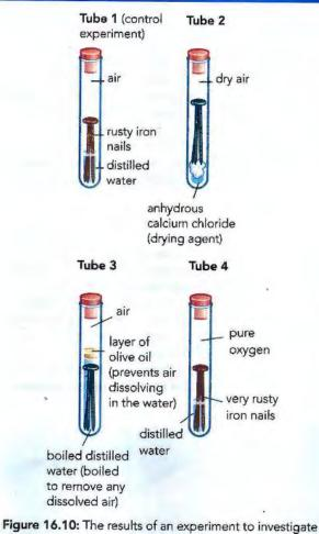
Figure 10.10: The results of an experiment to investigate the factors that are involved in rusting. In tube 2, the air is dry, so the nails do not rust. In tube 3, there is no oxygen in the water, so the nails do not rust. In tube 4, pure oxygen and water are present, so the nails are very rusty.
