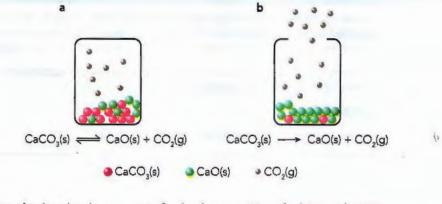
Figure 9.6: Comparison of a closed and open system for the decomposition of calcium carbonate.
