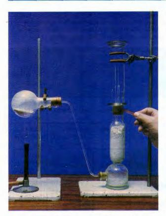
**Figure 11.8:** Preparation of ammonia. The gas is dried by passing it through a tower containing quicklime (CaO). Note that ammonia turns red litmus blue.
