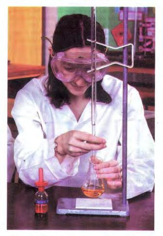
Figure 22.13: Performing an acid–base titration using methyl orange as indicator.
