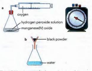
Figure 8.14 a: Apparatus for the experiments on the decomposition of hydrogen peroxide to water and oxygen. b: The black powder does not disappear during the reaction.
