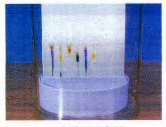
Figure 21.15: Separation of mixtures of inks by paper chromatography.
