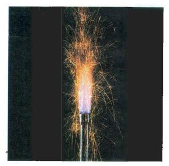
Figure 14.5: Iron dust ignited in a Bunsen flame.
