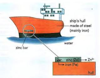
Figure 16.12: Blocks of zinc (or magnesium) are used for the sacrificial protection of the hulls of ships.
