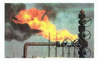
Figure 19.4: Excess natural gas (mainly methane) is sometimes flared off at oilfields.
