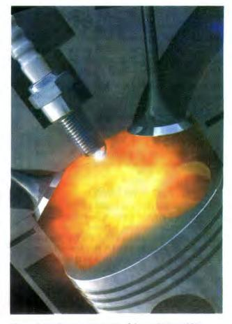
**Figure 8.11:** Computer graphic of the explosion within the cylinder of a petrol engine as the piston compresses the gases.
