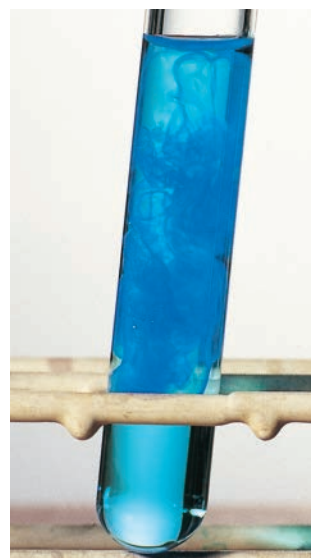
b Copper(II) hydroxide is precipitated
