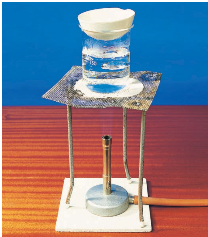
▲ Figure 8.8 The solution of magnesium nitrate is concentrated by slow evaporation
