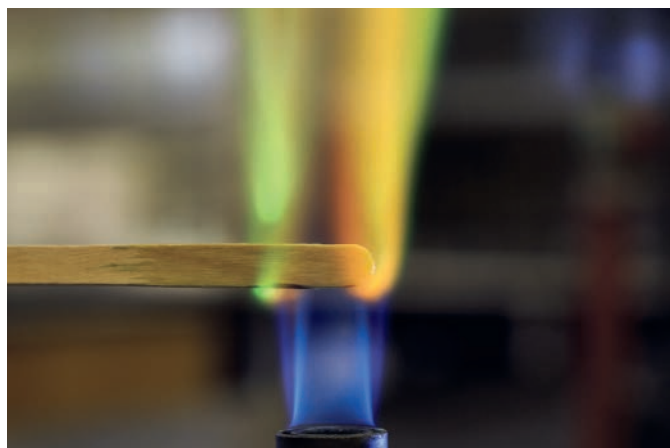
▲ Figure 14.27 The green colour is characteristic of copper
