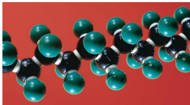
b Model of part of a PTFE polymer chain
