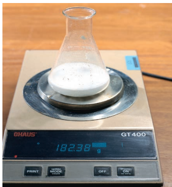
▲ Figure 7.4 After 60 seconds the mass has fallen by 1.24 g
