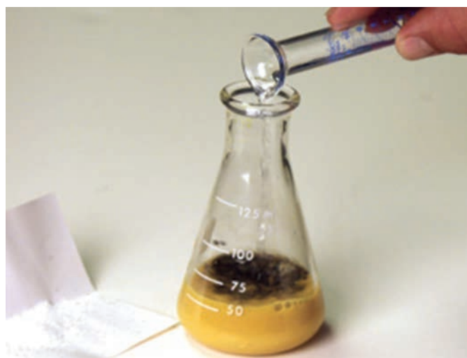
▲ Figure 3.11 The blue-black colour shows the presence of iron(III) ions
