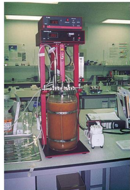
▲ Figure 18.5 A laboratory fermenter for antibiotic production, which will eventually be scaled up to 10 000-litre fermentation vessels
