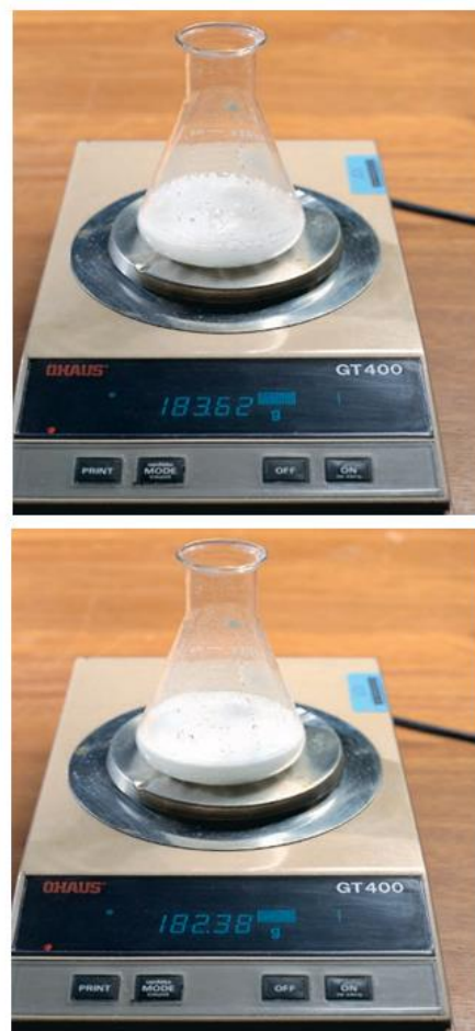
Figure 7.4 After 60 seconds the mass has fallen by 1.24 g
