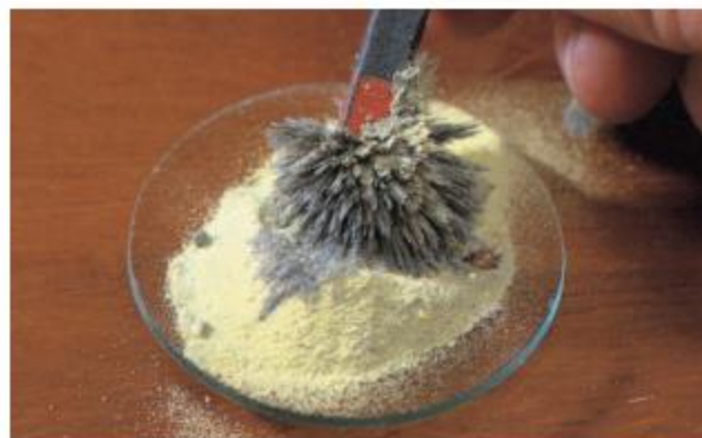
▲ Figure 2.9 A magnet will separate the iron from the mixture
