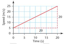
The gradient of the graph represents the rate of change of speed with time. The graph is a straight line, so the speed is changing at a constant rate.
