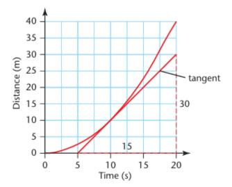
The graph is curving upwards, so the speed is increasing. You can estimate the speed of the object at a given time by drawing a line which touches the curve at that point. This is called a tangent.
