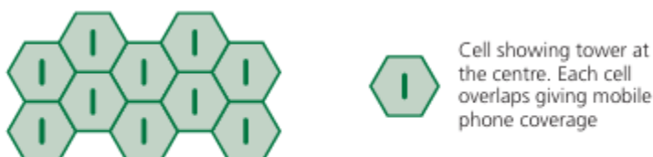
▲ Figure 6.4 Each cell overlaps, giving mobile phone coverage.
