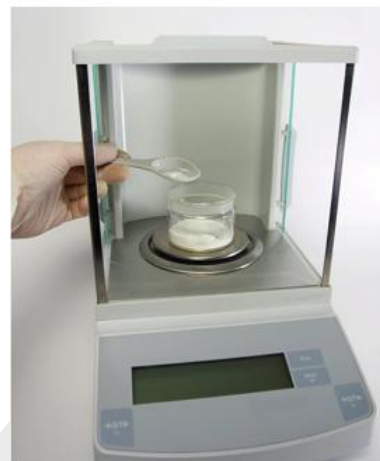
fig A This balance is tared (set to zero) and ready to use. The pan is enclosed; this is necessary on a four-decimal place balance because of fluctuations in the reading caused by draughts of air.
