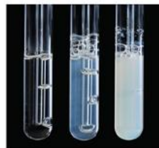
fig A As carbon dioxide is bubbled through limewater, the amount of precipitate increases.
