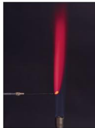
fig A A platinum wire loop with a sample of a strontium compound being held in a Bunsen flame.
