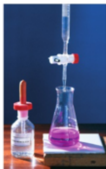
▲ fig C This shows the burette after the titration has been done. Note the white tile and the colour of the phenolphthalein indicator. The pink colour shows that an acid has been neutralised and there is an excess of an alkali.
