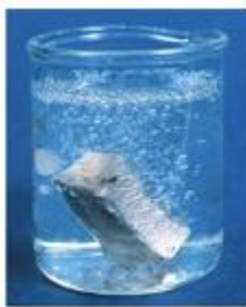
▲ fig D Calcium reacting vigorously with water.
