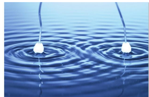
▲ fig C When waves meet, the displacements would add to each other to give the overall displacement for each location.
