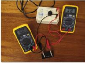
▲ fig A Measuring the resistance of an ohmic conductor.
