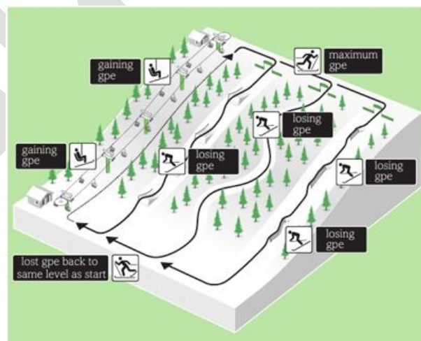
fig C Modelling an electric circuit as a ski area.
