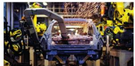
▲ Figure 15.10 Mild steel is used for car bodies . . .
