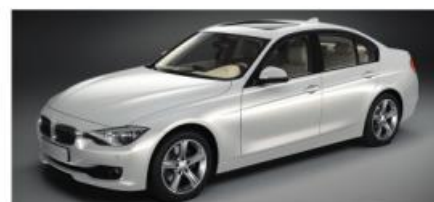
▲ Figure 15.11 Some cars have a body made of aluminium. In this photo the car body has been painted. The paint is mainly for decoration; it is not required to prevent rusting.
