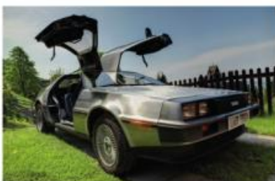
▲ Figure 15.13 Some cars have a stainless steel body. They do not need to be painted.
