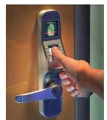
▲ Figure 1.51 A fingerprint scanner detects unique patterns in your fingerprints
