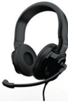
▲ Figure 1.48 This headset contains a microphone and headphone speakers
