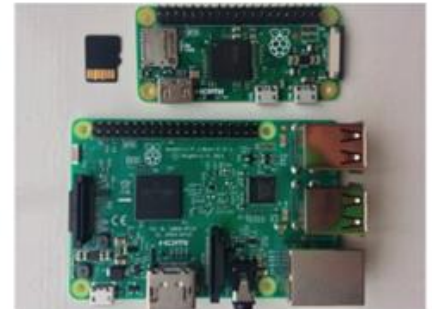
▲ Figure 1.6 The Raspberry Pi Zero (top) and its microSD card (top left)
