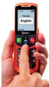
▲ Figure 1.8 The Alto 2 'talking phone' reads the names of contacts and text messages aloud to its user
