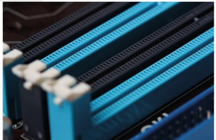
▲ Figure 3.2 A user can increase the amount of RAM using RAM slots on a motherboard
