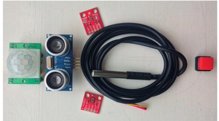
▲ Figure 1.59 (Left to right) motion sensor, proximity sensor, temperature sensor and button sensor; the red item at the top is a light sensor and the red item at the bottom is a UV sensor
