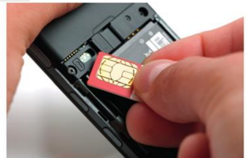
▲ Figure 1.7 The SIM card from a mobile phone
