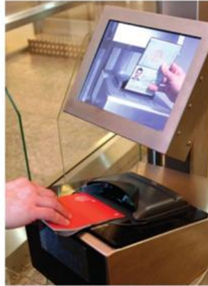
▲ Figure 1.55 Some passports now contain a chip that holds biometric data about the passport holder that is compared with the results of biometric scans carried out at airports
