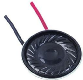
▲ Figure 1.70 A piezoelectric 'piezo' speaker used in a watch
