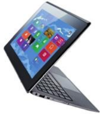
▲ Figure 1.22 Some laptops now have touch screens that can flip 360 degrees, allowing them to operate as tablet devices
