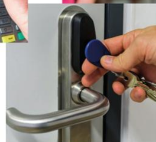
▲ Figure 1.58 RFID tags can be included in a variety of objects
