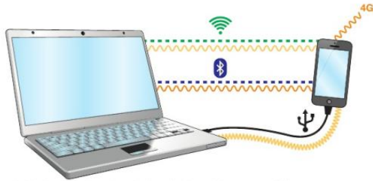
▲ Figure 4.6 Devices can be tethered using wired or wireless connectivity
