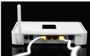
▲ Figure 5.12 This router has a four-port switch; the last (grey) port on the right is used to connect the router to a WAN (in this case, the internet)
