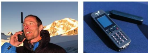
▲ Figure 4.11 Satellite telephones use antennae to transmit data to (and receive data from) one or more satellites
