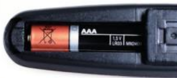
▲ Figure 7.6 When one coulomb of charge passes through this cell it gains 1.5 J of energy.
