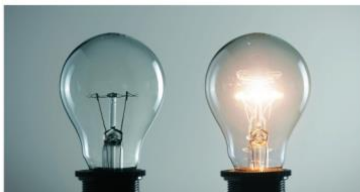
▲ Figure 6.11 It is the heating effect of a current that is causing this bulb to glow.
