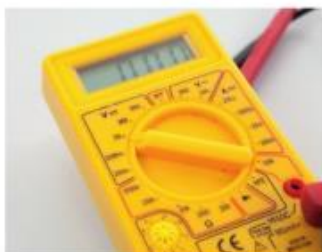
▲ Figure 7.8 A voltmeter measures voltages across a component.
