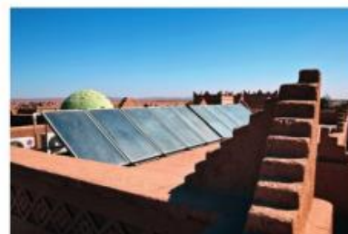
▲ Figure 15.12 Shiny and white surfaces reflect thermal radiation, while matt black surfaces, like in the solar heating panels, absorb it.
