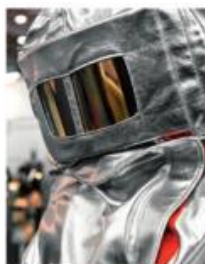
▲ Figure 15.12 Shiny and white surfaces reflect thermal radiation, while matt black surfaces, like in the solar heating panels, absorb it.
