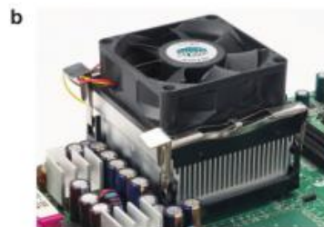
▲ Figure 15.13 a A shiny kettle stays warmer longer. b The heat sink needs to be matt black to lose heat to the surroundings quickly, and so stop the transistor overheating.
