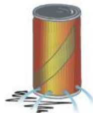
▲ Figure 18.6 Pressure in liquids acts equally in all directions. A can of water with holes can be used to demonstrate this.
