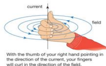
▲ Figure 20.10 You can work out the direction of the field using the right-hand grip rule (for fields).
