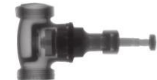
▲ Figure 24.4 A gamma camera image used to view inside a valve
