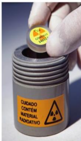
▲ Figure 24.9 Radioactive samples are stored in lead-lined containers and are handled with tongs or protected fingers.
