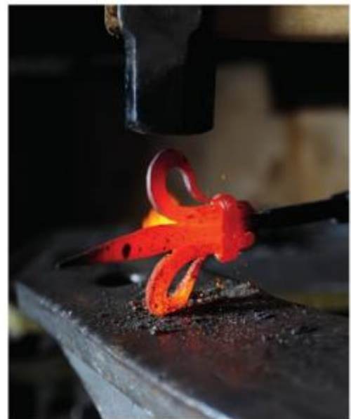
▲ Figure 27.4 The colour of the light emitted by this piece of iron tells us how hot it is.
