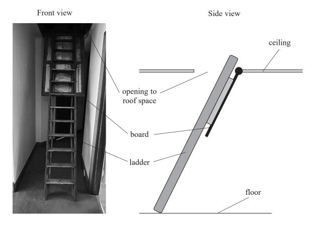
When not in use, the ladder is stored in the roof space and the opening to the roof space is covered by a board. The board is hinged to the ceiling at one end.
