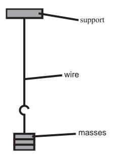
The wire broke when the extension was small.
