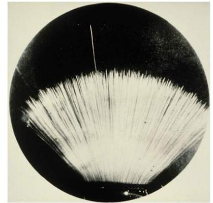
**Figure 16.17** Alpha-particle tracks show up in this photograph of a cloud chamber. Notice that all the particles travel roughly the same distance through the air, indicating that they all have roughly the same initial kinetic energy.
