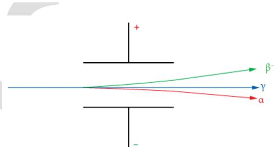
**Figure 16.15** An electric field can be used to separate  $\alpha$ -,  $\beta^-$ - and  $\gamma$ - radiations. (The deflection of the  $\alpha$ -radiation has been greatly exaggerated here.)
