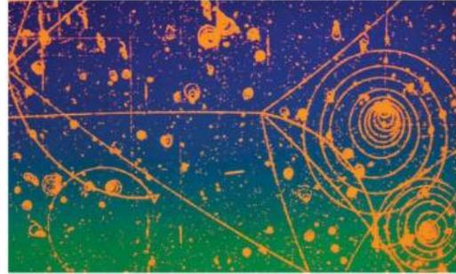
**Figure 16.9** Particle tracks in a bubble chamber detector. A particle has entered from the left and then struck another particle just to the right of the centre. Four new particles fly out from the point of impact.
