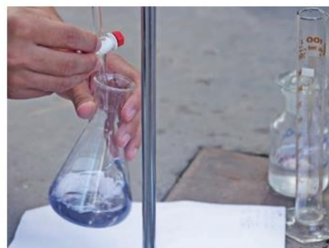
▲ Figure 8.9 The acid is added to the alkali until the indicator just changes colour
