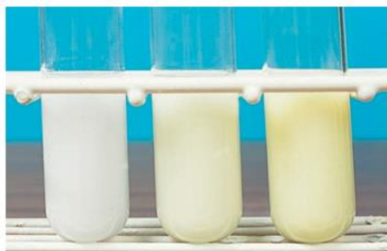
▲ Figure 8.14 AgCl, a white precipitate, AgBr, a cream precipitate, and AgI, a yellow precipitate
