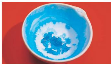
▲ Figure 8.11 After slow evaporation to concentrate the solution, the solution is left to crystallise. Crystals of copper(II) sulfate are produced
