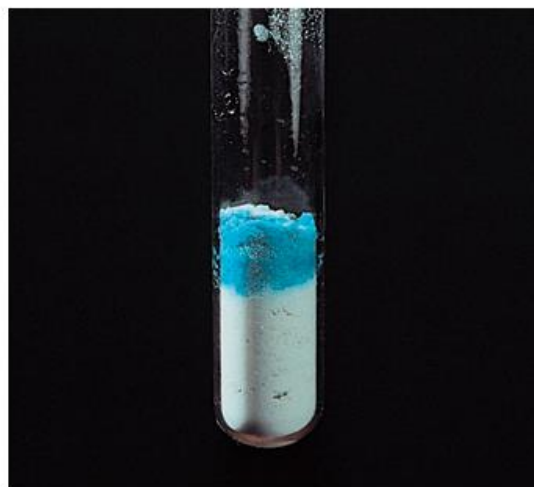
▲ Figure 8.16 Anhydrous copper(II) sulfate is a white powder which turns blue when water is added to it
