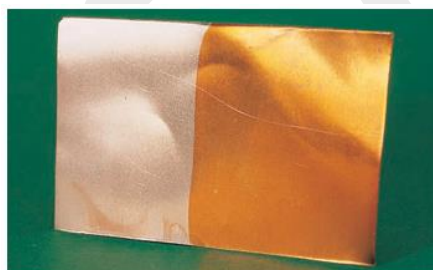
▲ Figure 8.10 Citric acid has been used on the right-hand side of this piece of copper metal to remove the oxide coating on its surface. The acid reacts with the oxide coating to form water, leaving shiny copper metal
