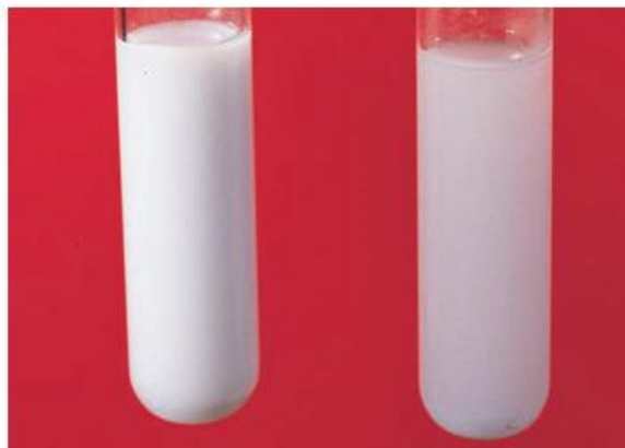
▲ Figure 8.13 If left to stand the white precipitate of silver chloride goes grey. This photochemical change plays an essential part in black and white photography
