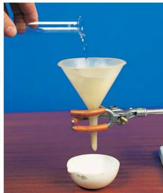
▲ Figure 8.7 The excess magnesium is filtered in this way
