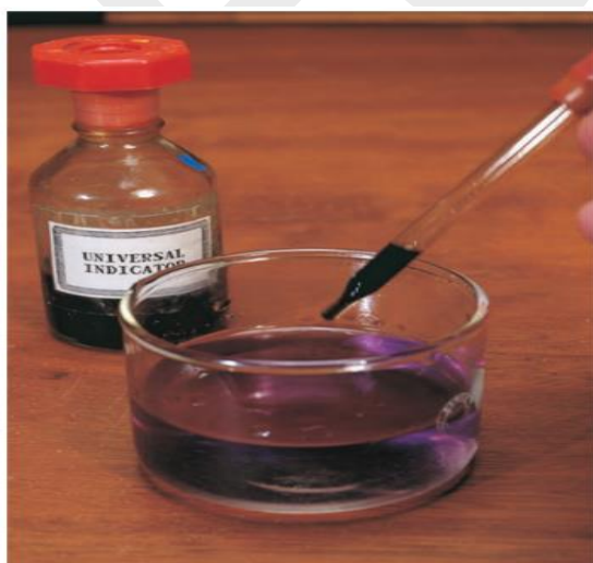
b An alkaline solution is produced when potassium reacts with water
