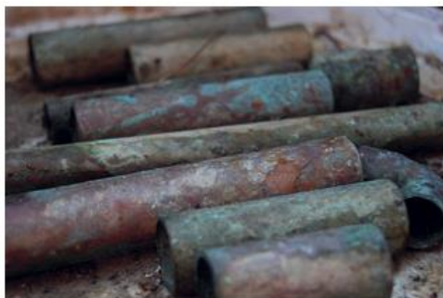
▲ Figure 10.23 Verdigris soon forms on the surface of copper materials in exposed environments
