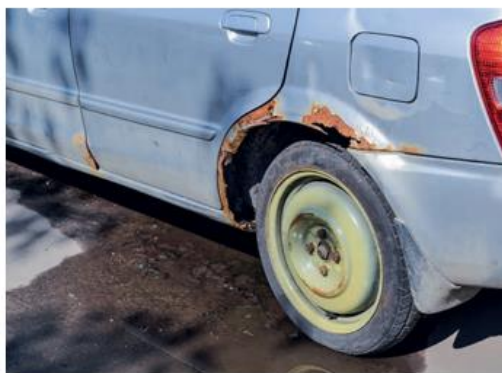
▲ Figure 10.19 A brand new car is protected against corrosion (top). However, if the paintwork is damaged, then rusting will result
