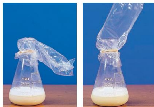
▲ Figure 13.8 Fermenting glucose and yeast to produce ethanol. The bag is inflated during the experiment by CO 2
