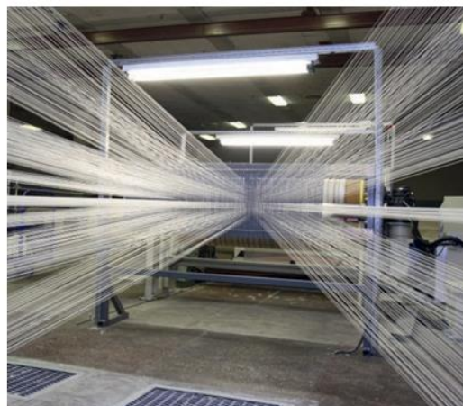
▲ Figure 13.12 Nylon fibre is formed by forcing molten plastic through hundreds of tiny holes
