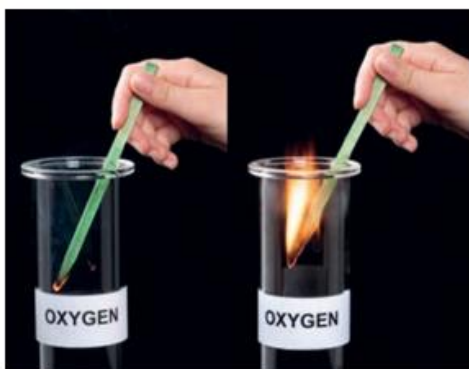
▲ Figure 14.31 Testing for oxygen gas
