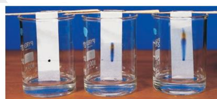
a Chromatographic separation of black ink
