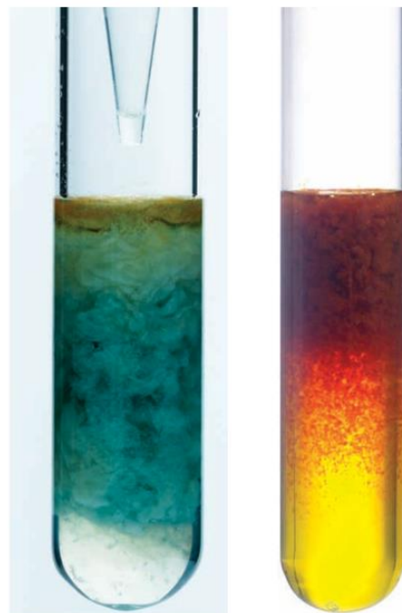
▲ Figure 14.28 Addition of sodium hydroxide will show the difference between \text{Fe}^{2+} and \text{Fe}^{3+} in aqueous solution
