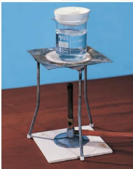
▲ Figure 14.12 Apparatus used to slowly evaporate a solvent
