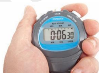
▲ Figure 14.1 This stopwatch can be used to measure the time passed in a chemical reaction. The reading is 6.3 s
