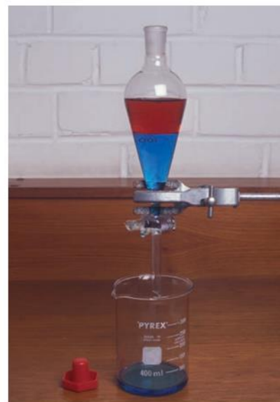
▲ Figure 14.17 The blue liquid is more dense than the red liquid and so sinks to the bottom of the separating funnel. When the tap is opened the blue liquid can be run off.
