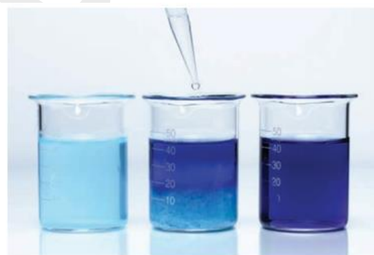
▲ Figure 14.29 When aqueous ammonia is added to a solution containing \text{Cu}^{2+} ions the solution forms a gelatinous light blue precipitate. As more is added to excess, the precipitate dissolves, forming a dark blue clear solution
