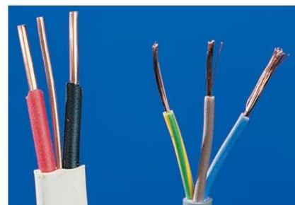
a The copper used in electrical wiring has to be very pure
