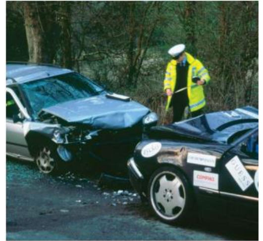
Figure 6.7 The front of each car has crumpled in, as a result of a head-on collision.
