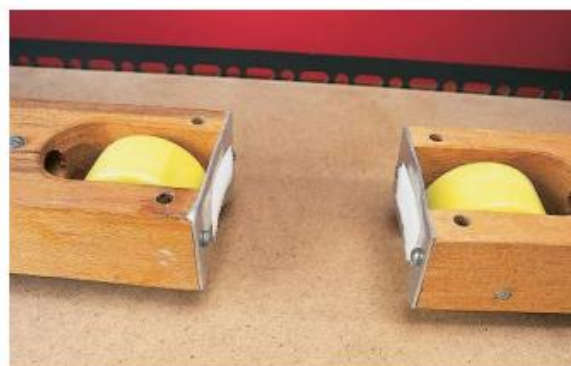
Figure 6.4 If a moving trolley sticks to a stationary trolley, they both move off together.
