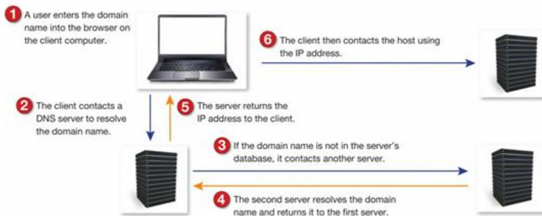
▲ Figure 5.8 Domain name service (DNS)
