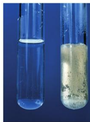
fig C Colour change of Tollens' reagent from a colourless solution to a silver mirror in the test for an aldehyde.
