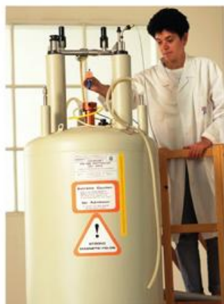
fig B The largest part of NMR equipment is often the large vacuum flask containing liquid helium, needed to cool the magnets to below 4 K.
