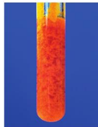
fig C This is the bright orange precipitate formed when a carbonyl compound reacts with 2,4-dinitrophenylhydrazine.
