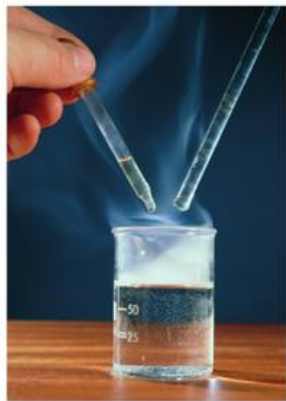
fig A Adding ethanoyl chloride to water produces fumes of hydrogen chloride.
