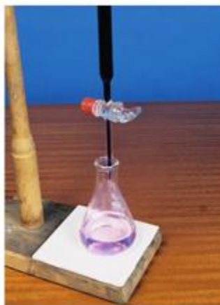
▲ fig A End point colour in a potassium manganate(VII) titration.
