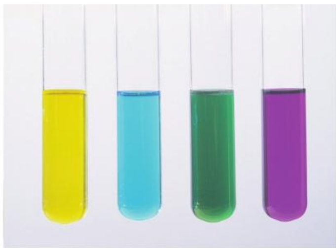
▲ fig A The tube on the left (yellow) contains the VO_2^+ ion. The second tube (blue) contains the VO^{2+} ion. The third tube (green) contains the V^{3+} ion. The tube on the right (purple) contains the V^{2+} ion.
