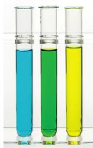
▲ fig C The pale blue solution contains [\text{Cu}(\text{H}_2\text{O})_6]^{2+} , the yellow solution on the right contains [\text{CuCl}_4]^{2-} and the green solution in the middle contains a mixture of the two.
