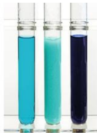
▲ fig B The pale blue solution contains [\text{Cu}(\text{H}_2\text{O})_6]^{2+} , the pale blue precipitate contains [\text{Cu}(\text{H}_2\text{O})_4(\text{OH})_2] and the deep blue solution contains [\text{Cu}(\text{NH}_3)_4(\text{H}_2\text{O})_2]^{2+} .
