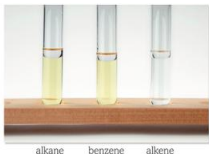
fig C The yellow colour is caused by unreacted bromine.
