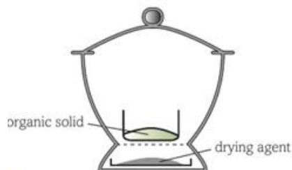
▲ fig B Drying an organic solid in a desiccator
